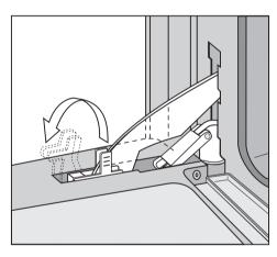
Holding the door evenly with both hands, lift the door up and off the hinges.
